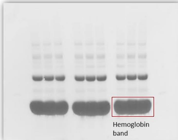
Figure Annex V. 1: Example of a membrane colored with Ponceau solution after transference. Hemoglobin band was used to normalize areas obtained from final WB results of RBC PRDX2 and PRDX SO 2/3 quantification using ImageJ software.
