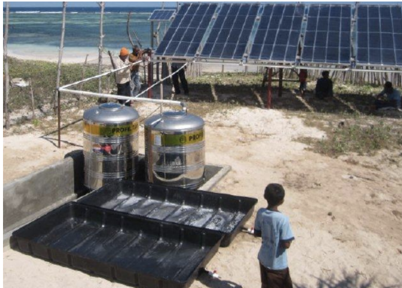
Figure 3.5 Example of a F CUBED installation with an open-air evaporator where salt crystallises. (Source: Solar Water Purifier – Water purification systems, 2022).
