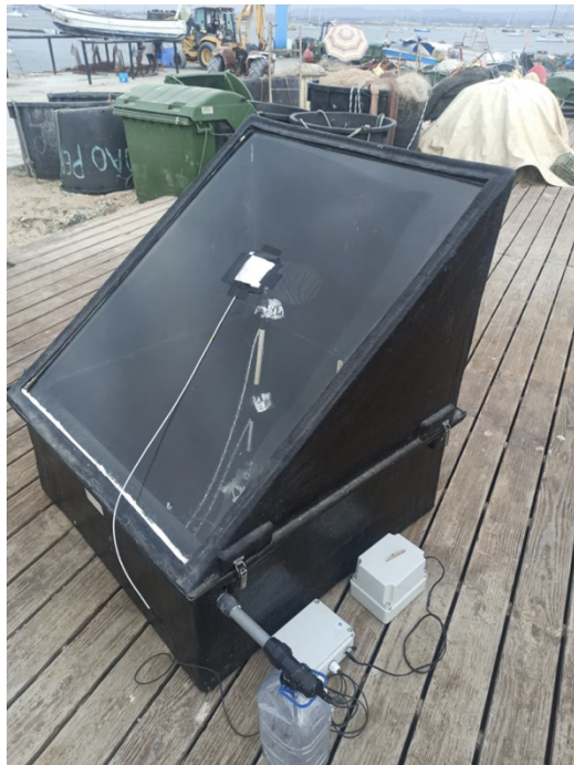
Figure 2.7 Solar still built by ROLEAR and installed on Culatra Island
