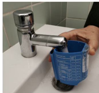
Figure 2.2 Water flow rate measurement in situ . (Source: Muller, 2019).
