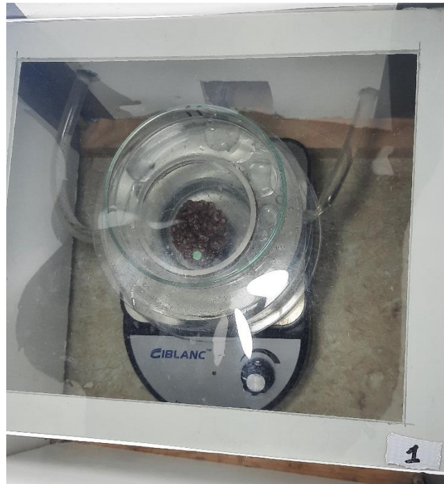
Annex Figure 2. (Left and Right) Open Acrylic incubation chamber, set on magnetic stirrer, with rhodolith being mounted. (Bottom) Closed Incubation Chamber with set Light Filter cover.
