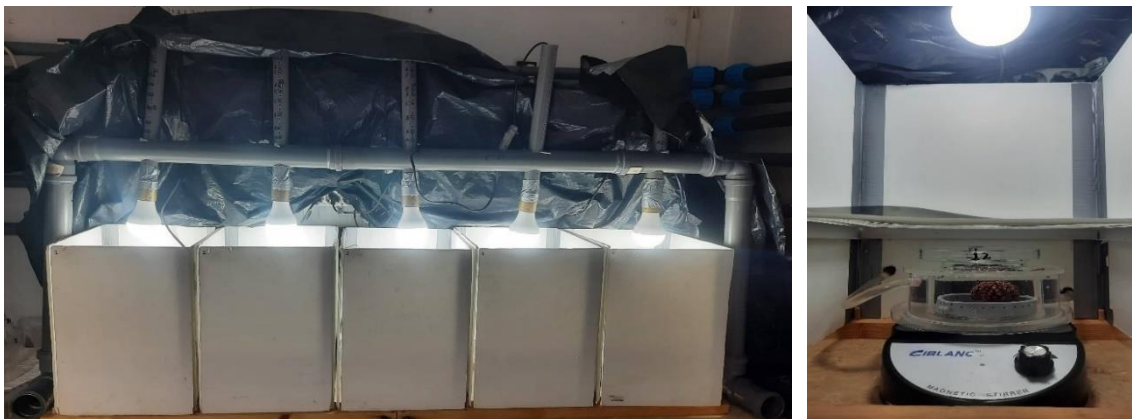
Figure 2.3.1. (Left) Set-up of 5 incubation chambers and regulating lights. (Right) Acrylic incubation chamber, set on magnetic stirrer, holding a rhodolith. Light intensity is set by height of light bulb and covering filter (above chamber)
