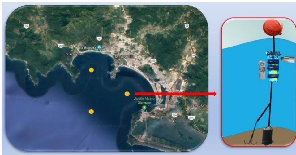
Figure 3.2. Map of the Manzanillo and Santiago Bays that shows the point of the location of the buoys. In the right, the structure with the hydrophone, the buoy, the plastic container with acoustic equipment, and the anchor used in each sampling site.
