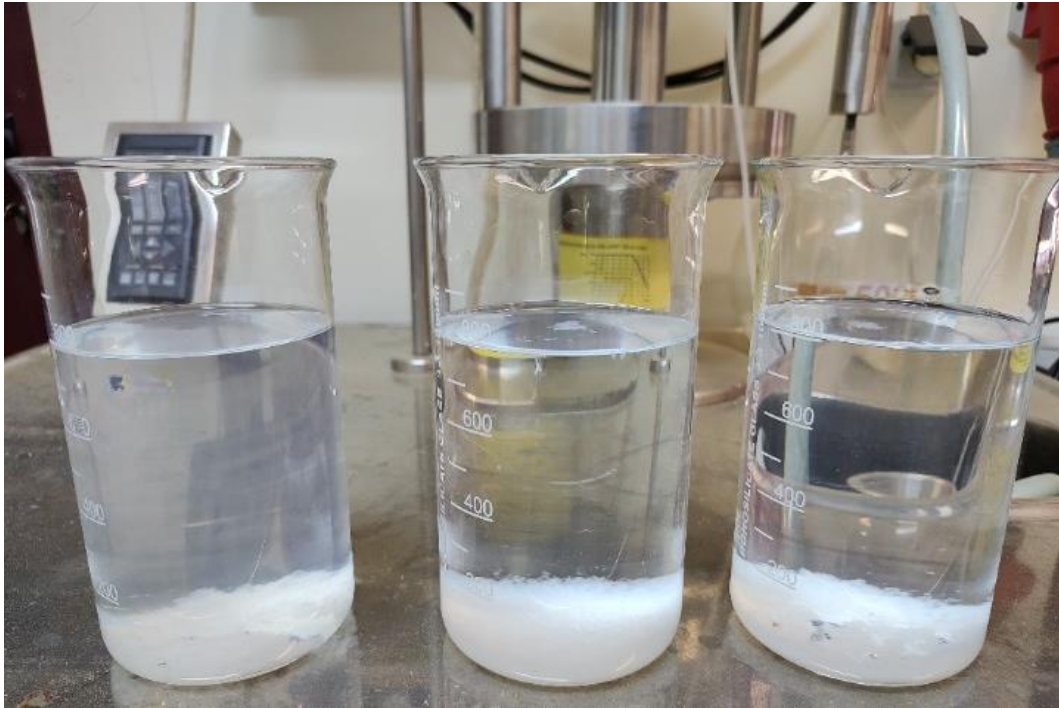
Figure 3.24: Turbidity removal after coagulation/flocculation test using commercial coagulant
