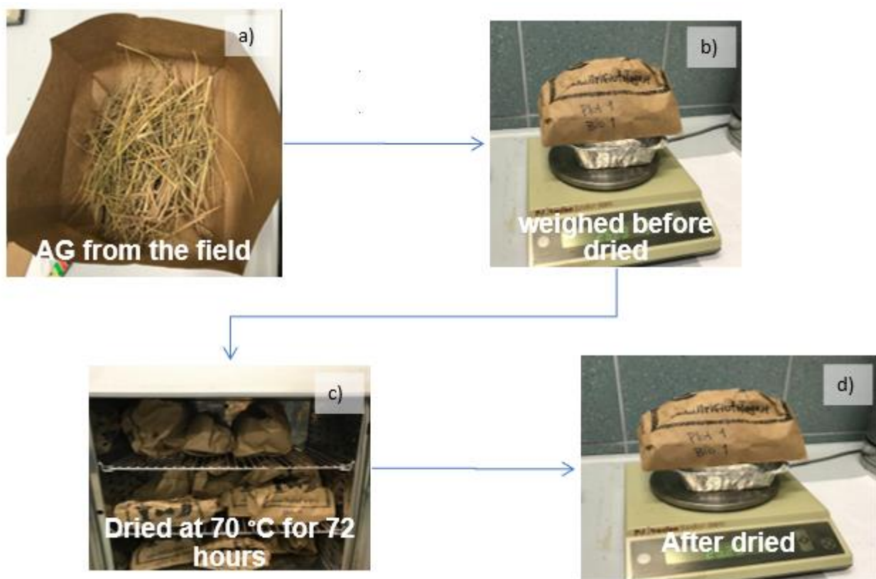
Figure 2-6 Laboratory process for the above ground biomass
