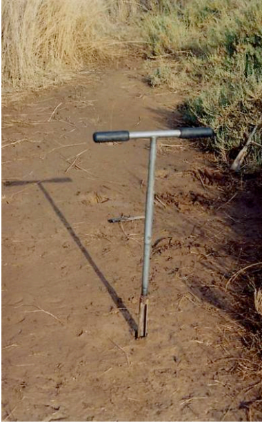
Figure 3. Half-cane hand corer apparatus which has a diameter of ca 3 cm.
