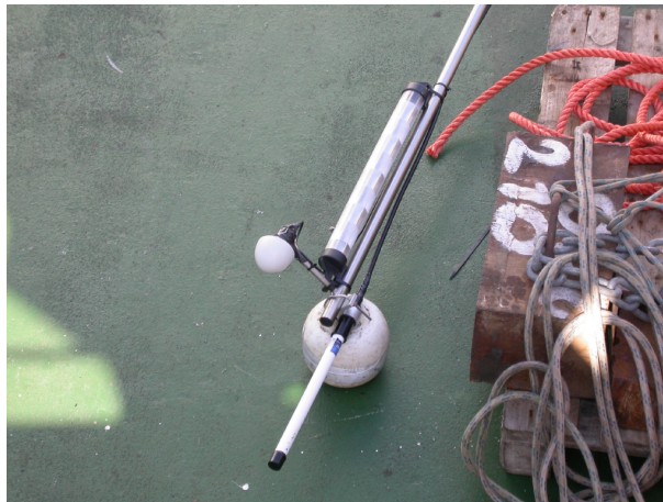
Figure 2.3: Acoustic Oceanographic Buoy mast: GPS cone antenna, wireless lan monopole and radar reflector (long transparent tube below the antennas).
