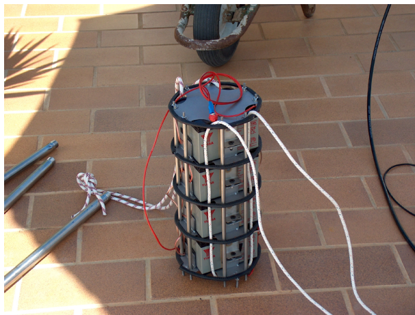
Figure 2.5: Acoustic Oceanographic Buoy battery pack.
