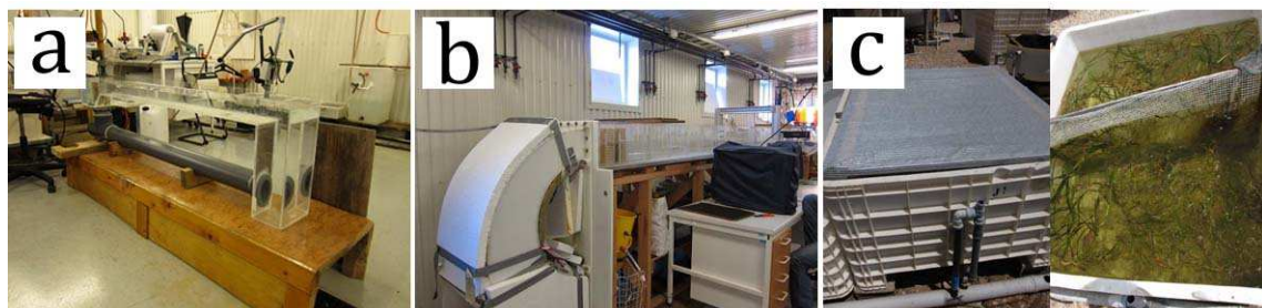
Figure 2.2. Flume tanks used to quantify (a) dispersal potential of Zostera noltii seeds and (b) damage of fragments occurring during exposure to currents, both in the biohydrodynamic laboratory of Sven Lovén Centre for Marine Sciences – Tjärnö, University of Gothenburg. (c) View of uncovered and covered outdoor tanks for still water experiments of the dispersal potential of vegetative fragments, in Ramalhete field station, University of Algarve.
