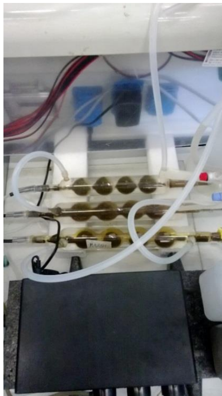
Fig. 2.3: Up-flow anaerobic sludge blanket (UASB) reactor used for experiment
