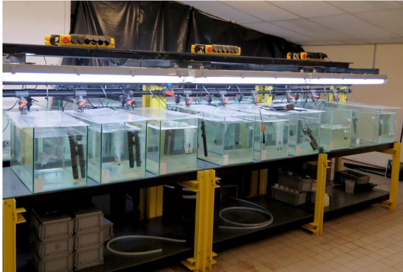
Fig. IV.2: Experimental set up, showing the tanks, water and air supply, at IFREMER facilities.
