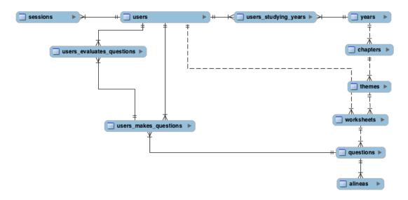
Figure 1. Relational database structure to support the mobile application
