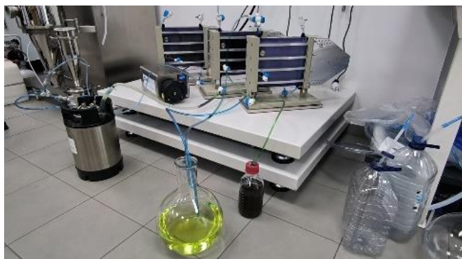
Figure 3.16: Experimental setup utilized for the membrane filtration fractionation assay.
