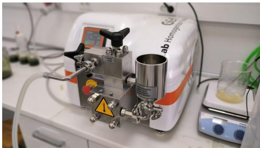
Figure 3.10: Experimental high pressure homogenization setup utilized to perform the HPH optimization assay.
