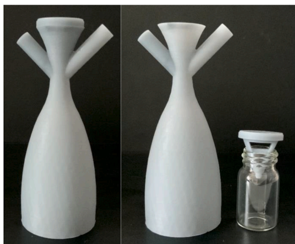
Fig. 3. Prototype printed by stereolithography using UV light and a washable resin. On the left, the prototype is assembled, while on the right, both the main body and the weighing head are separated.
