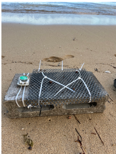
Figure 2.1: Double layer tray for experimental nama cultivation with weight stone and data logger
