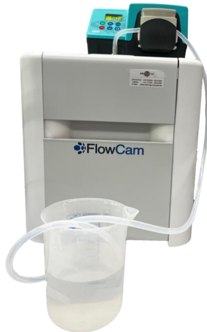
Figure 3: Flowcam setup with tubing and Peristaltic Pump
