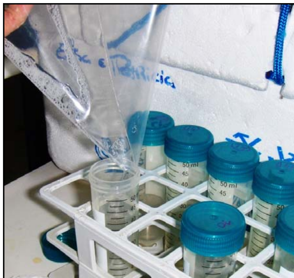
Figure 6. Transfer of mucus from the collecting bag to a 50 ml sterile centrifuge tube.
