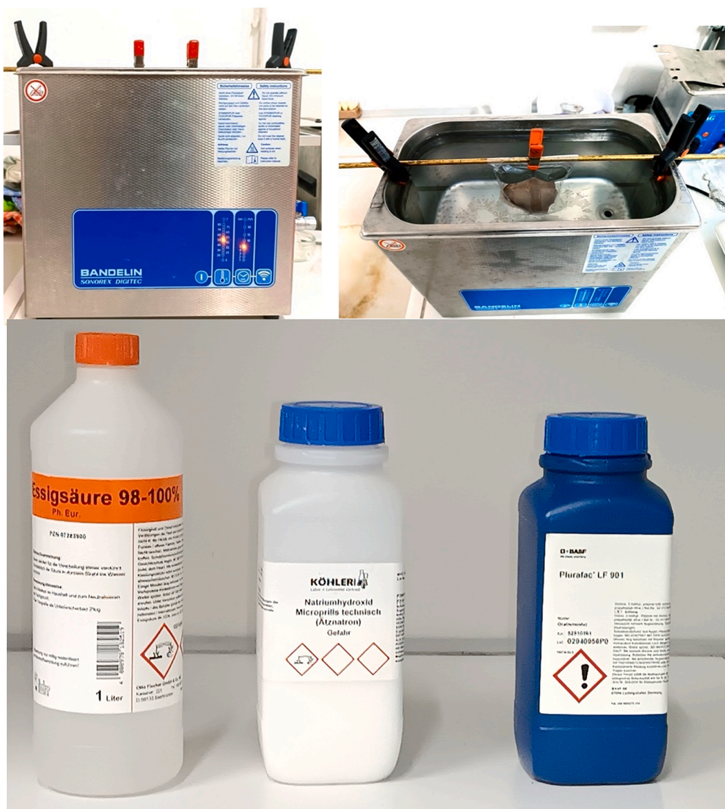
Fig. 5. Ultrasonic basin and the chemical products used for cleaning the experimental samples.
