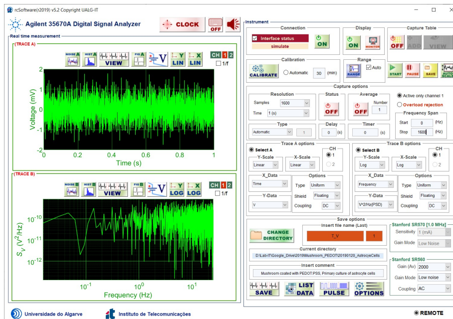
Figure 2.10: RC software application developed by Pedro Inácio (unpublished) for processing and visualizing data in real time.
