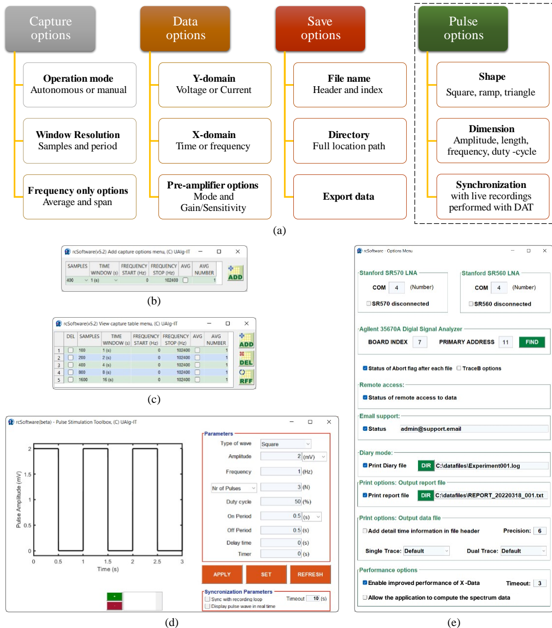
Figure A.3 – Programmable options and additional features provided through the DAT user interface to perform live and standard data logging. (a) Schematic representation of the main programmable options. Pulse options are delineated by a black dashed line to indicate that it's an optional feature. (b–e) GUI of the menus for adding and viewing the capture table options, the Pulse Stimulation Toolbox (PST), and the options menu DAT, respectively. The PST is still under development (a beta version).
