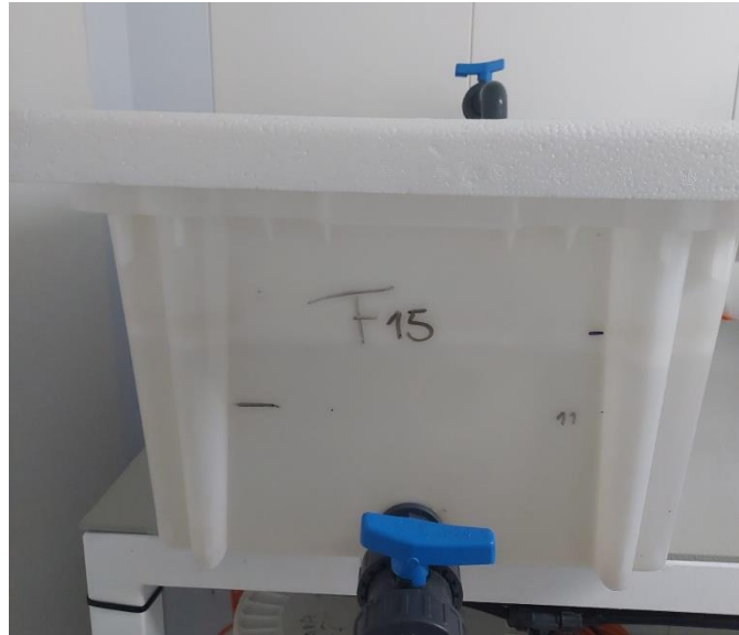
Figure 3.2. Infection tank with a styrofoam cover to prevent contaminations of other experiments
