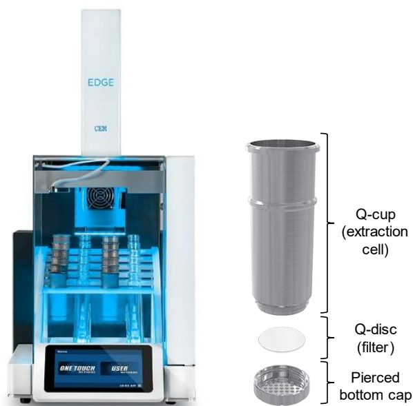
Figure 8. EDGE extractor (left) and scheme of an EDGE extraction cell or Q-cup (right). Adapted from 41 .
