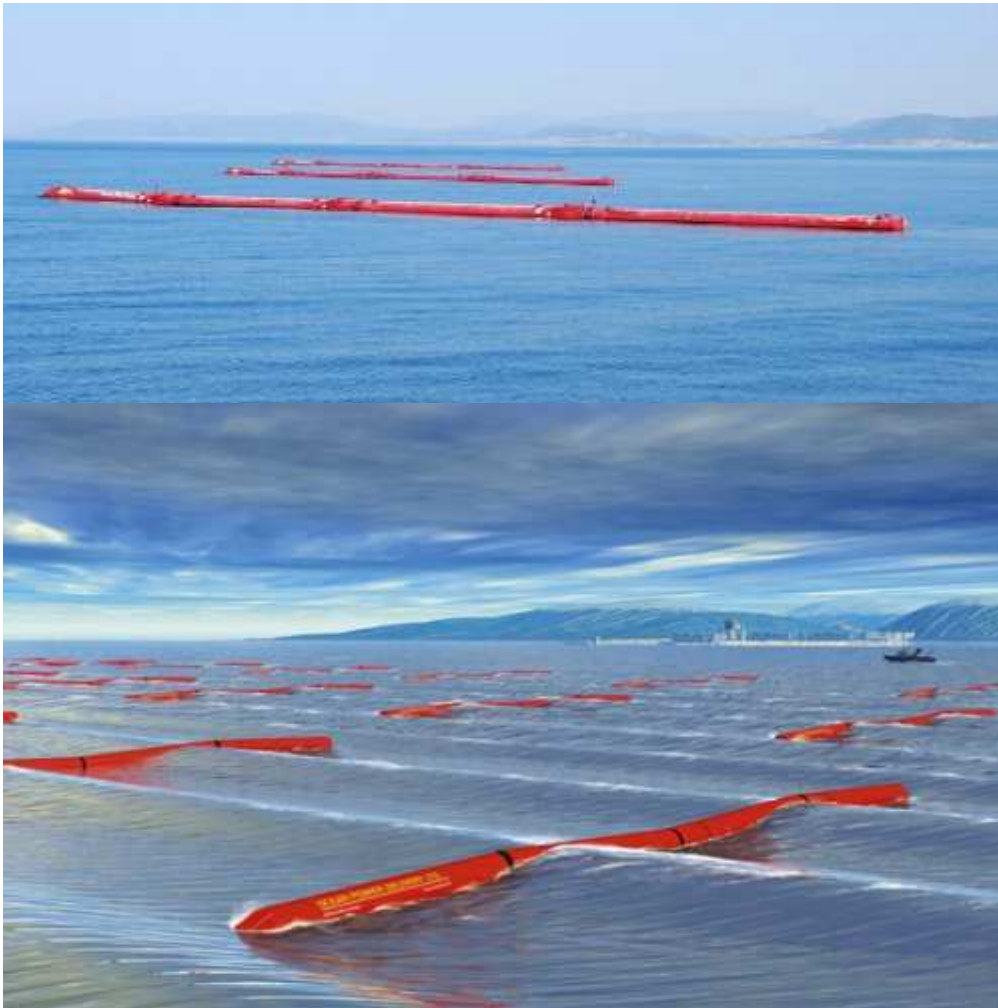
Fig 25. Pelamis wave farm. The upper side of image shows the current wave farm project (3 devices), and the lower shows the planned wave farm (21 devices). (Source: www.pelamiswave.com/ )
