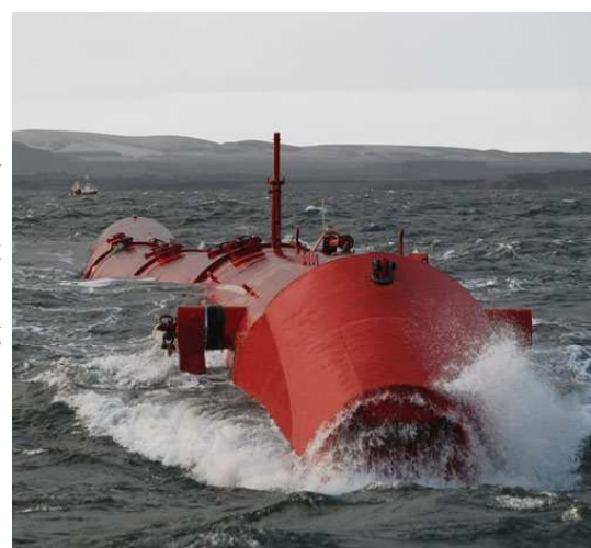
Fig 24. Pelamis device in off-shore location. (Source: www.pelamiswave.com/ )
