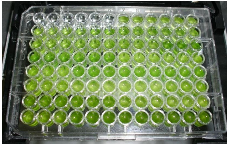
Figure 3.4 - 96-well plate containing algae culture from 5-L plastic bottles for spectrophotometry analysis.
