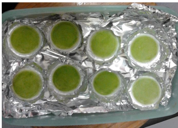
Figure 3.6 - Glass microfiber filters (VWR, 1.2 \mu\text{m} ) containing 10 mL of algal culture and dried for 72 hours
