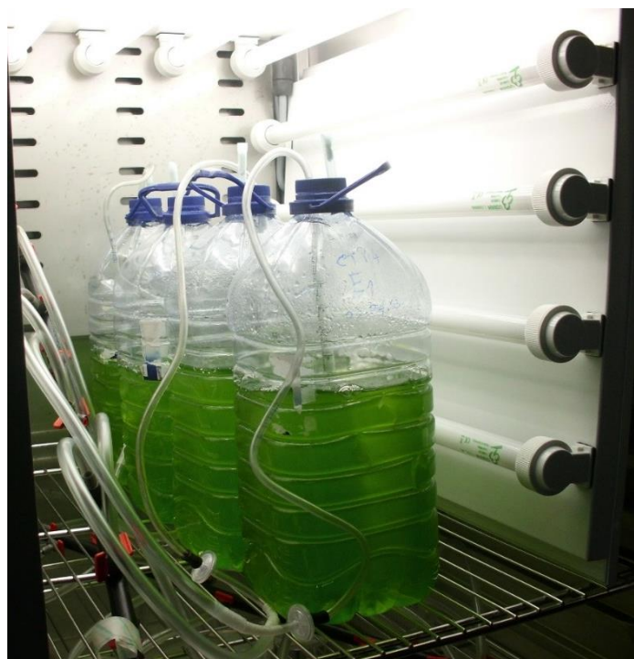
Figure 3.1- CTP4 cultivation in 5-L plastic bottles under continuous air flow at control conditions to establish growth correlations.
