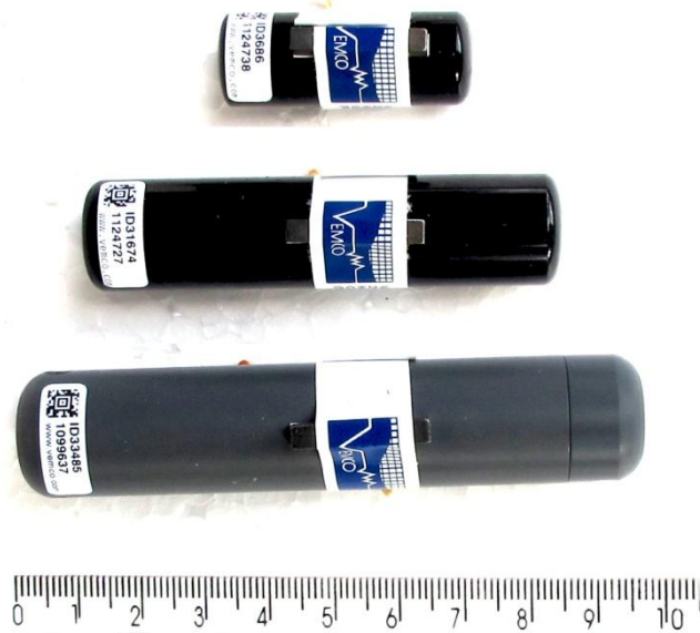
Figure SUP.7.3. Aspect of the coded, acoustic transmitters used for monitoring tiger shark movements, namely V13 (top) and V16 (middle) transmitters for surgical implantations and V16 transmitter with shark-case (bottom) for external attachment. Scale is in centimeters.
