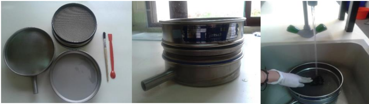
Figure 2.6: Sediment granulometry by the sieving process for evaluating the coarse grain ratio.
