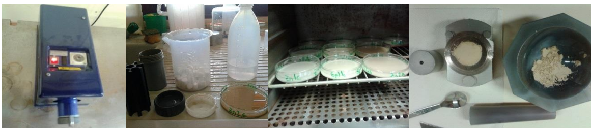
Figure 2.8: The figure shows the process carried out for each sample for mineralogical analysis as described in the text, namely: the grinding equipment, the two containers and resulting wet fine sediment, the drying petri dishes in the oven and the agate mortar.
