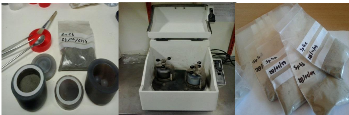
Figure 2.9: Homogenization process using a ball mill (FRITSCH, planetary micro mil, pulverisette 7): Agate containers with balls (left), ball mill equipment (center), resulting powders (right).
