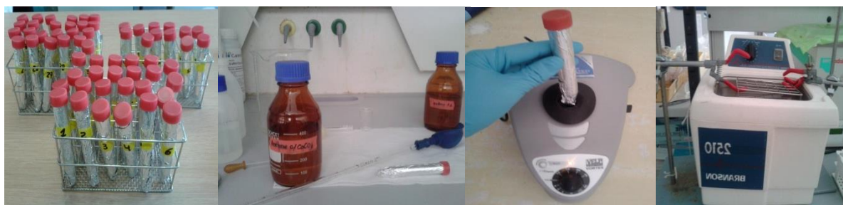
Figure 2.11: Pigment extraction process: samples protected against direct light (first image), acetone addition (second), vortex (three) and sonication process (fourth).
