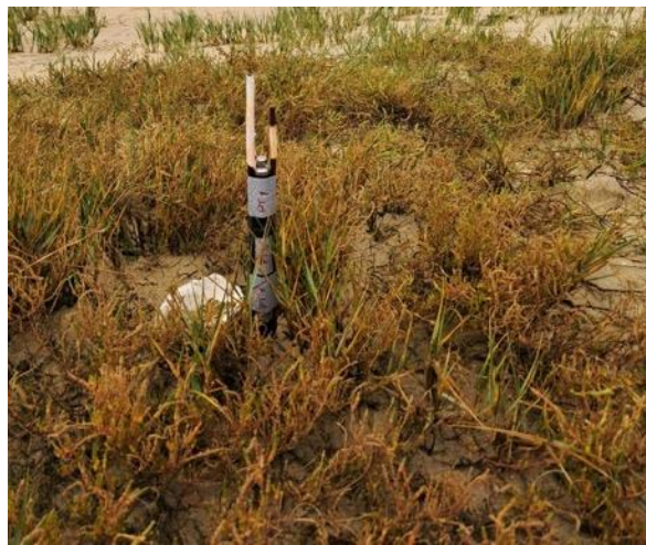
Figure 6. Installation of a Pressure transducer (PT) to measure water depth (example of deployment at the low marsh in S2 profile).
