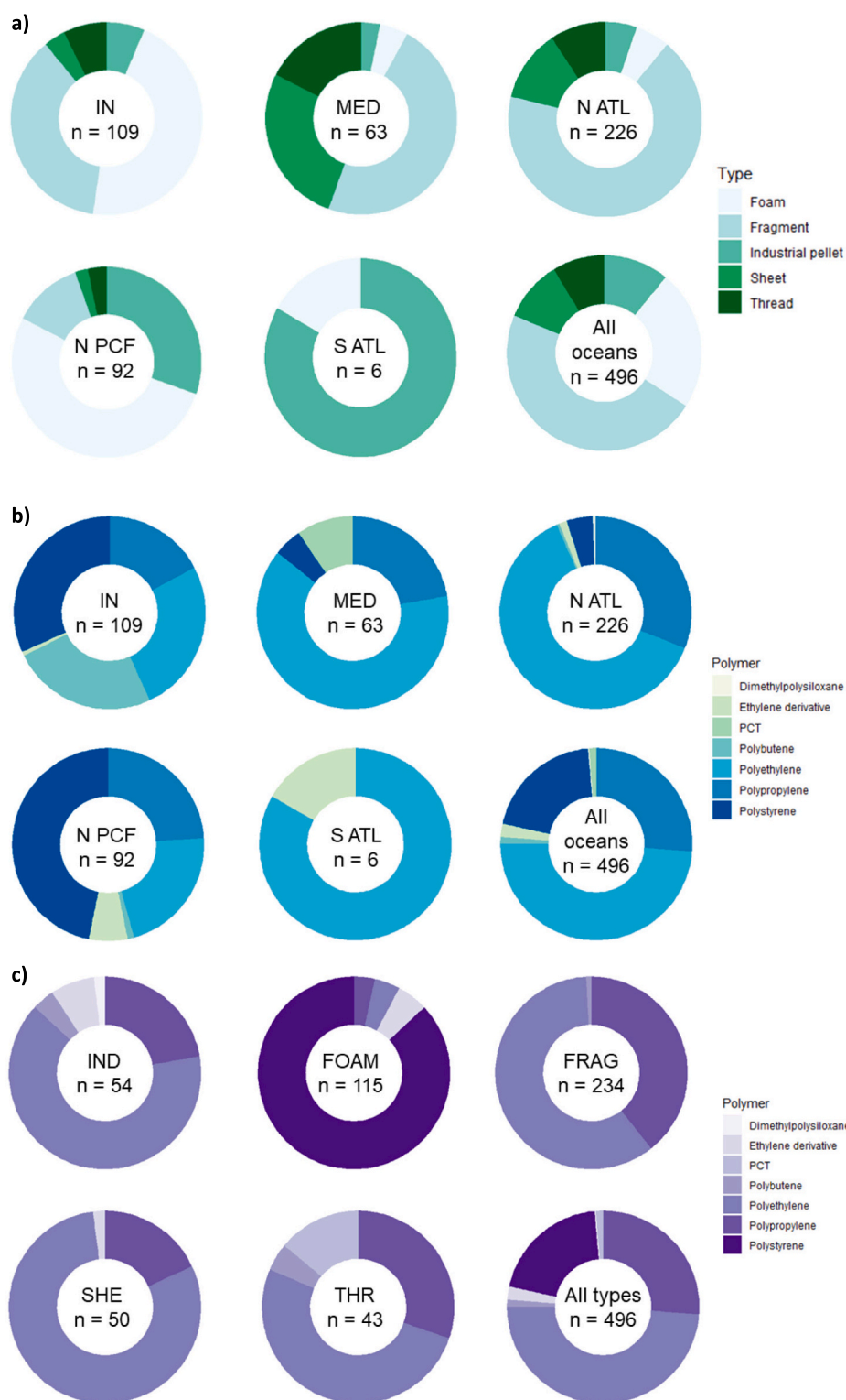
Fig. 3. a) Composition of large microplastic (1–5 mm) types by ocean basins. b) Composition of large microplastic (1–5 mm) polymers between oceans (IN = Indian, MED = Mediterranean, N ATL = North Atlantic, N PCF = North Pacific, S ATL = South Atlantic). PCT = Polycyclohexylenedimethylene terephthalate. c) Composition of large microplastic (1–5 mm) polymer by microplastic type (IND = Industrial plastic pellets, FOAM = Foams, FRAG = Fragments, SHE = Sheetlike plastics, THR = Threadlike plastics).
