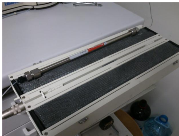
Figura 13 - High-Performance Liquid Chromatography Elite LaChrom Hitachi
