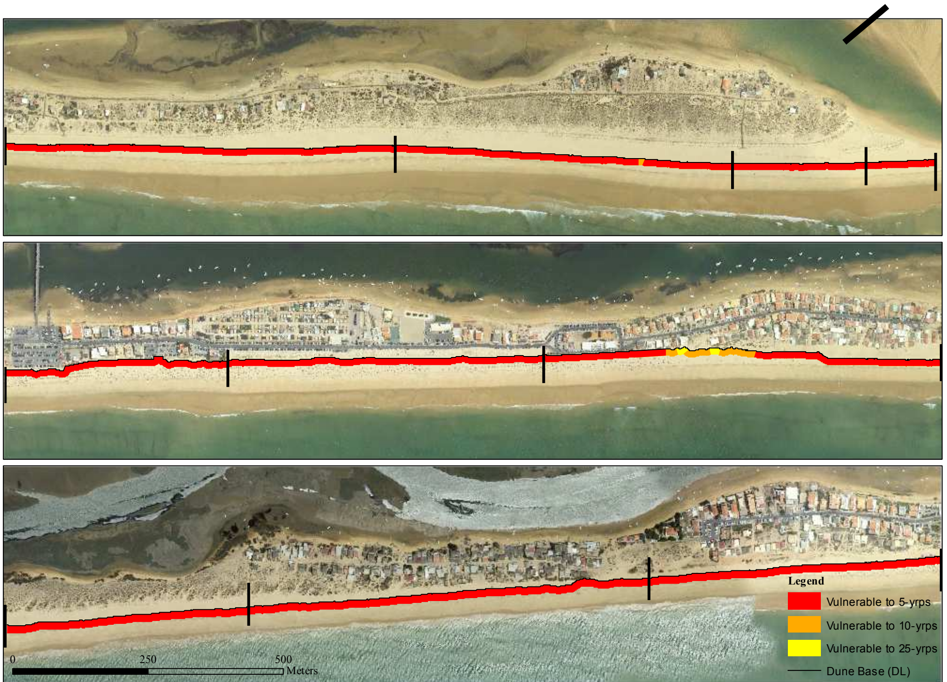
Figure 12 – Representation of collision regime vulnerability along the study area for 5, 10 and 25 – year return period storm.
