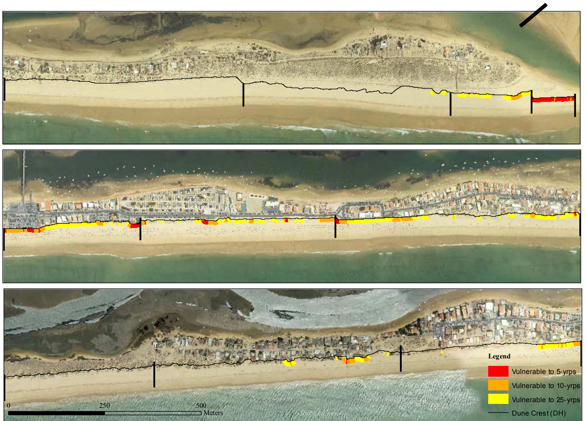
Figure 10 – Representation of overwash regime vulnerability along the study area for 5, 10 and 25 – year return period storm.
