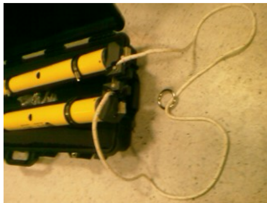
Figure 3.6: Using two Releasers in parallel
