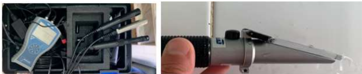
FIGURE 14. ODEAN RANGE PROBE (LEFT) AND HANDHELD REFRACTOMETER (RIGHT)
