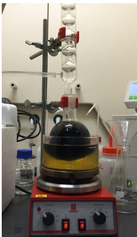
Figure 4.3 - Transesterification of the lipids to produce the biodiesel.
