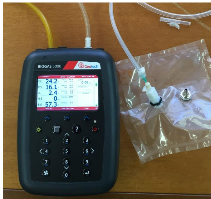
Figure 4.7 - Measurement of the biogas composition with a Geotech Biogas 5000.
