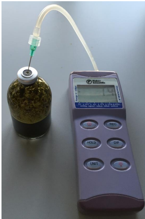
Figure 4.6 - Measurement of the pressure on the head space to estimate the biogas production.
