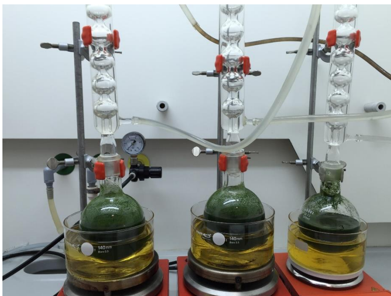
Figure 4.2 - Extraction of the lipids from the B. braunii biomass.
