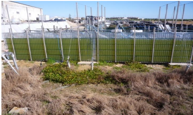
Figure 4.1 - Green wall airlift photobioreactor at NECTON S.A. facilities (Pereira, 2009).
