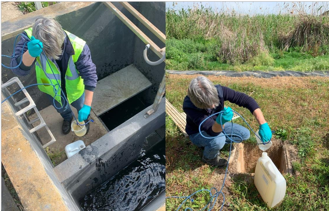
Figure 3.1. Águas do Algarve, S.A. staff using a sampler cup to collect effluent from Carrapateira (left) and Maria Vinagre (right) WWTP.
