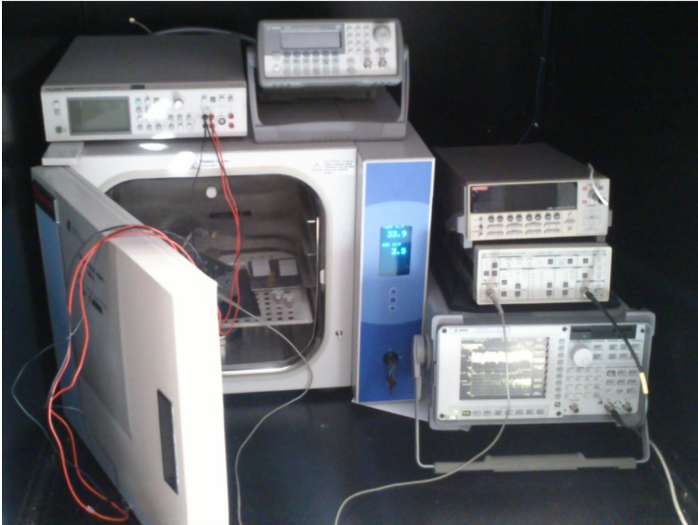
Figure 4.3 Photograph of the experimental set-up used for electrophysiological measurements. The photo shows the view of the instruments placed inside the Faraday cage. The cell incubator, a dynamic signal analyser and a low noise voltage amplifier.
