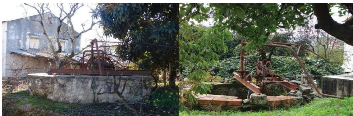
Figure 6. Examples of animal-driven irrigation devices using engineered pump (authors).
