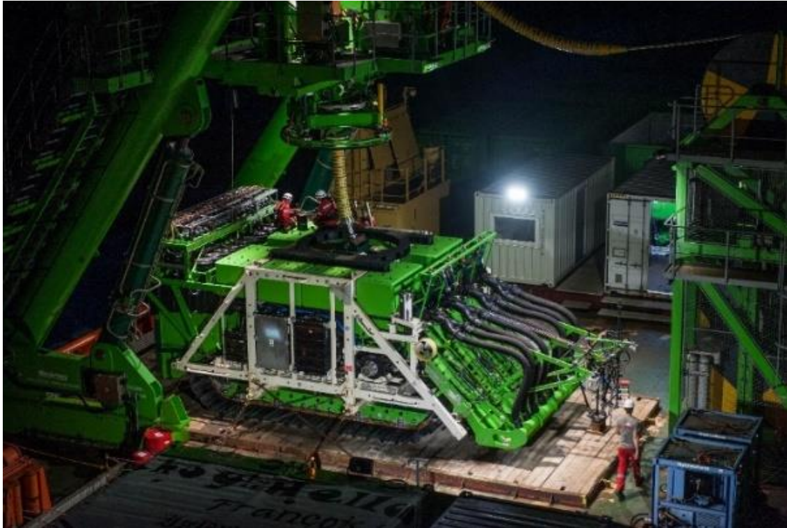
Fig.2.2- Pre-prototype nodule collector, Patania II, used to simulate a small-scale mining activity on the BGR and GSR contract areas of the CCZ. Source: © GSR
