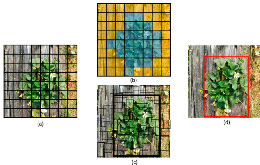
Figure 4. Detection steps of the YOLO model. (a) Input image with an N \times N grid, (b) class probability prediction map, (c) bounding box prediction for each grid, and (d) the detection result.
