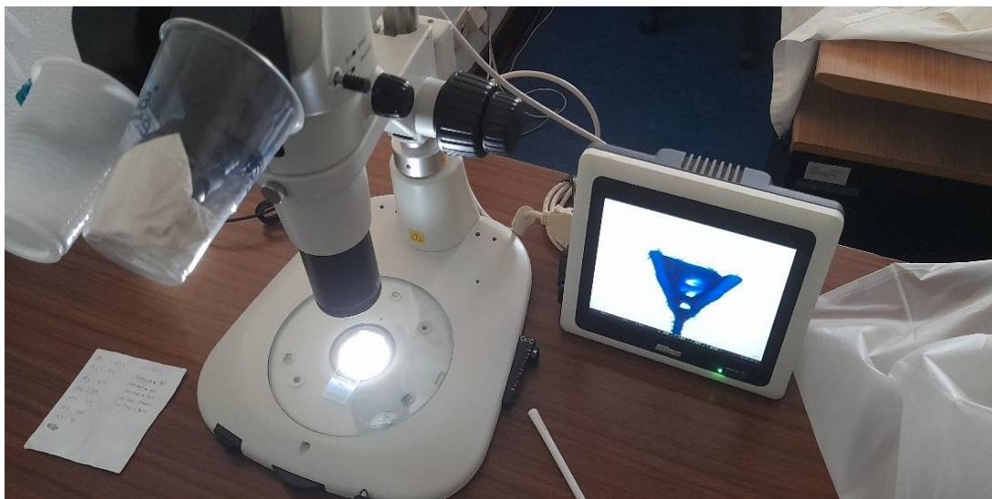
Figure 2.7 – Nikon P-DSL32 dissecting microscope used to visualize vertebral sample slides of longfin mako sharks ( I. paucus ) and Nikon Digital Sight DS-L3 camera and screen for image and scale adjustments.
