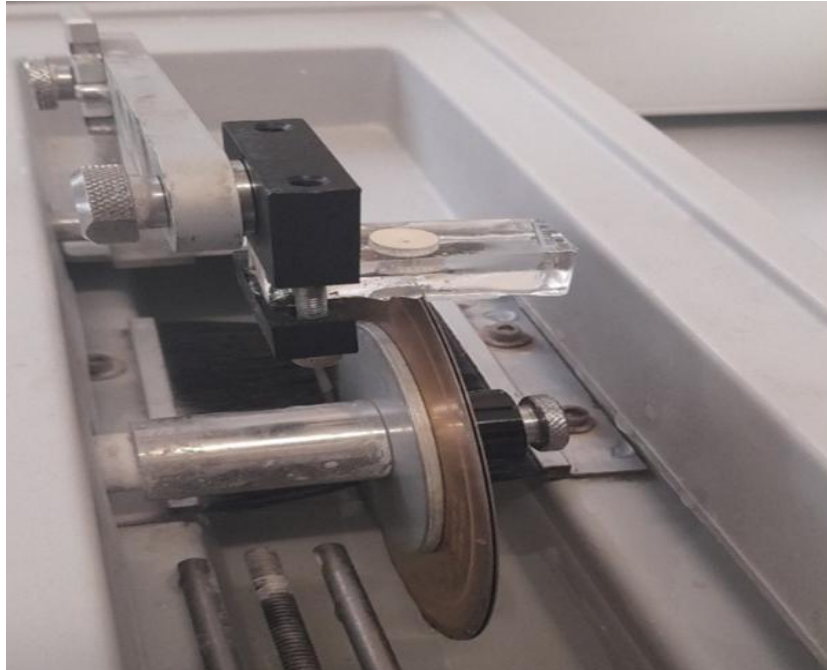
Figure 2.5- Buehler Isomet model low-speed saw, equipped with two diamond wafering blades. The lower chamber of the machine was filled with water to keep the blade tips wet, performing a centered 0.3 mm sagittal section of the longfin mako shark ( I. paucus ) vertebra.
