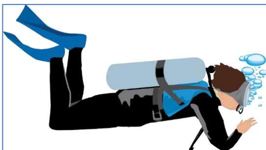
Figure 4: Schematic presentation of the trim position for most efficient buoyancy control. The body is in a horizontal Position. Ankles and knees are bend in an 90° angle. Arm remain free to perform tasks while diving. (Figure courtesy of Integration and Application Network ( ian.umces.edu/media library )).
