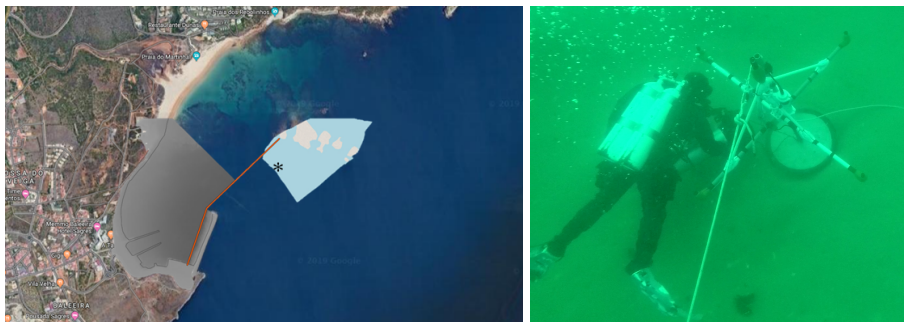
Fig. 1. The MARREAL Experimental setup in Sagres, off the Baleeira port: observatory deployment area; the position is marked by the * (left); acoustic system during the deployment (right).
