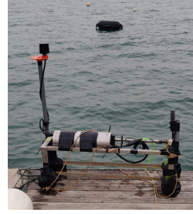
Fig. 3: Spiral source and underwater container near the anchorage site at the Lagoon.
