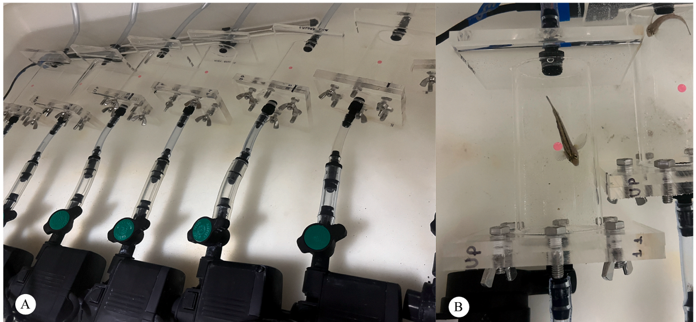
Fig. 4. Photos of the experimental set up of intermittent-flow respirometry chambers during O_2 measurement days. (A) Photo of the water bath with all respirometry chambers. (B) Close-up photo of one of the respirometry chambers used during the experiment.
