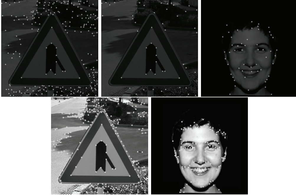
Figure 3.8: Top: results of automatic scale selection, without scale stability (left) and with stability over 20 scales (center and right). Bottom: results obtained with the SUSAN algorithm [Smith and Brady, 1997].
