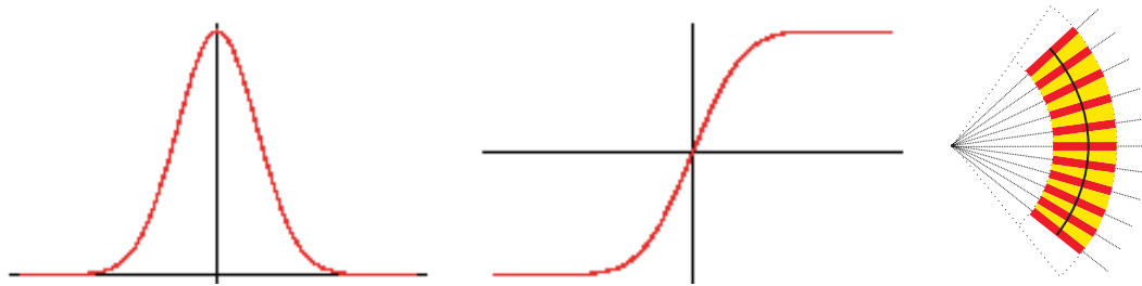
Figure 6.1: Left to right: 1D Gaussian line and errorfunction edge profiles, and the mapping and interpolation to obtain 2D profiles (see text).
