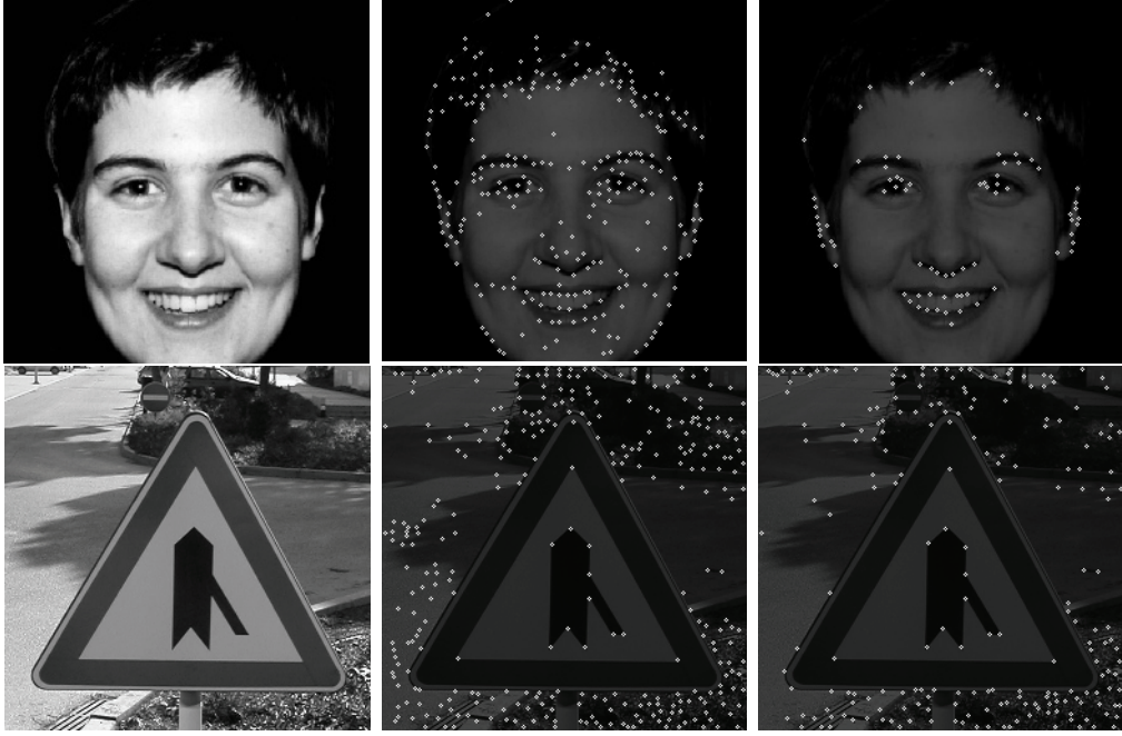
Figure 3.2: Keypoints detected at the finest scale, without (center) and with (right) NCRF inhibition.
