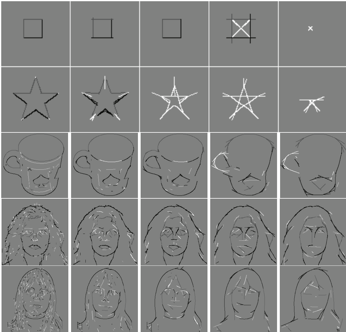
Figure 4.5: Top two rows: multi-scale line/edge representations of a square and a star at, from left to right, \lambda = \{4, 12, 18, 24, 40\} . Bottom three rows: a mug and two faces at \lambda = \{4, 8, 12, 24, 28\} .
