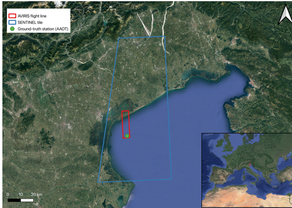
Figure 4: Study area showing the imagery tiles downloaded, including multi- (blue) and hyperspectral (red) imagery, and the ground-truth sampling station (green) for LoV.
