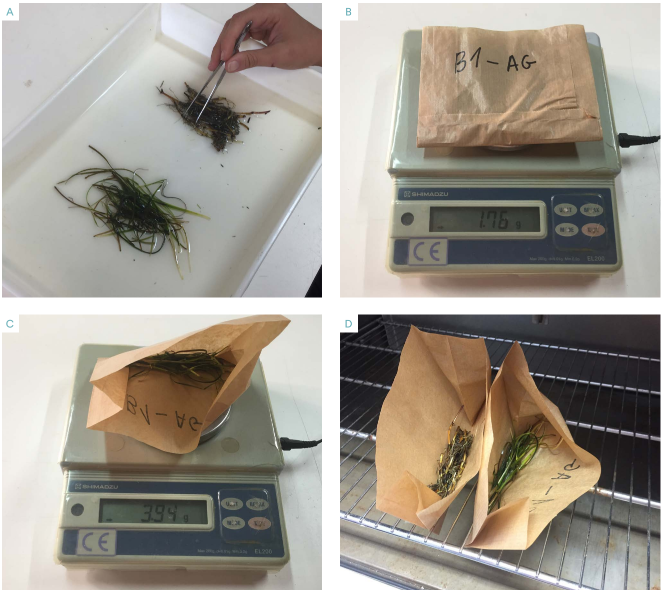
FIGURE 4.8. Pictures showing how a seagrass biomass sample is processed in the laboratory: A) separation of above-ground (leaves) and below-ground (rhizomes and roots) biomass, B) weighing the empty labelled paper bag before putting the biomass inside, C) weighing the paper bag with the biomass inside, D) drying the biomass in the oven. Photos by: C.B. de los Santos.
