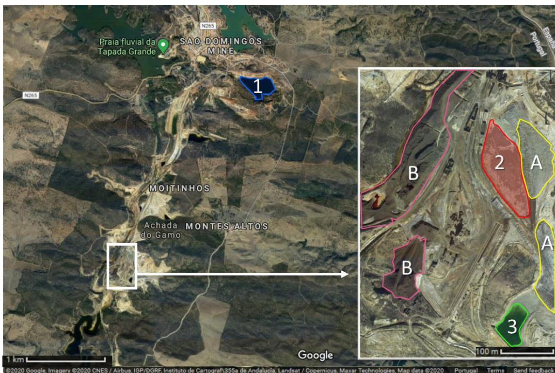
Figure 2.1. Aerial view of the the São Domingos mining area and a closer view of the sampled zone obtained from Google Maps: coordinates: 37°40'06.7"N 7°29'28.5"W. 1) Open pit mine; 2) Sampled impoundment with extreme acid mine drainage (AMD); 3) Another AMD impoundment; A) Roasted pyrite ore slag; B) Modern slag.
