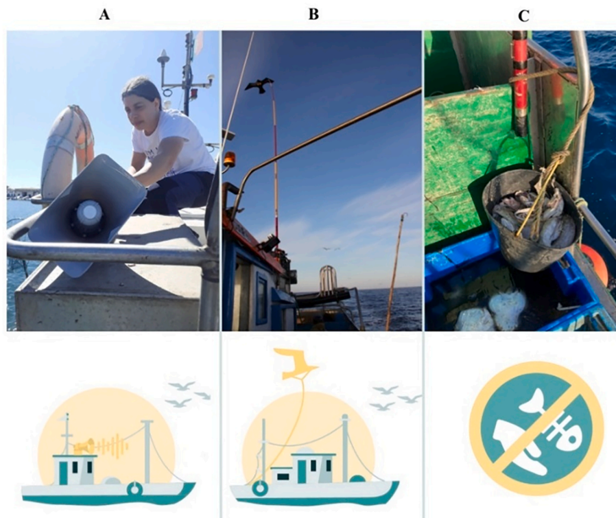
Fig. 2. (A) Megaphone implementation on a fishing vessel (top) and illustration of a fishing boat with the megaphone symbolizing the use of sound-based deterrents (below); (B) Scarybird implemented in a vessel (top) and illustration of a fishing boat with the scarybird representing visual deterrents (below); (C) Container strategically placed to the fishers, during net hauling and setting (top) and illustration representing the prohibition or management of offal discharge near fishing operations (below). Illustrations by Frederico Arruda. Photographs by Flávia Carvalho and Magda Frade.
