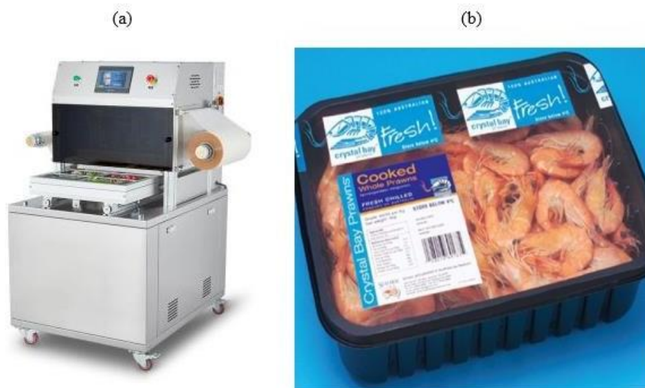
Figure 2.9 (a) A simple MAP machine (alibaba, n.d) (b) A typical modified atmosphere packaged seafood product (Worldfishing, 2015)
