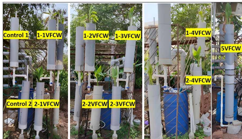
Figure 2 | Pilot-scale demonstrated two-stage vertical flow constructed wetland types.
